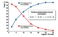
Phosphane ligands are observed to affect the addition of E-E bonds to alkynes: an excess of phosphane ligand decreases the performance of the catalytic reaction in some cases, whereas in others the catalyst is totally inactive in the absence of an excess of ligand. The metal particle leaching promoted by the phosphane ligand is used to create a new catalytic reaction.
