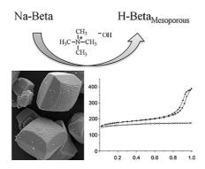
Zeolite beta was successfully desilicated using tetramethylammonium hydroxide. It is shown that calcination of the desilicated material directly produces the mesoporous acidic form of the zeolite. A protocol integrating the post-synthesis treatments desilication and ion-exchange is thus presented.
